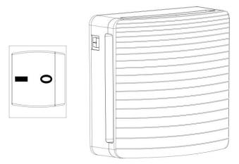
In case of one unit, turn on the product through "0/1" switch and then set a function by remote to activate the product accordingly. In case of more units, refer to paragraph "MASTER-SLAVE PRODUCTS CONFIGURATION" and, once this procedure is ended, turn ON the products through 0/1 switch and press a function by remote to activate the device.
